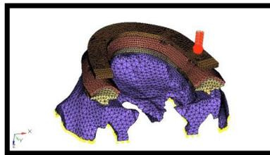
**Figure 6.** Load of 120 N applied vertically.
