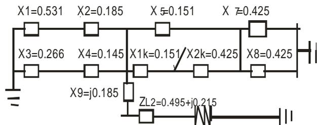
**Figure 4.0 System reverse sequence impedance diagram**
