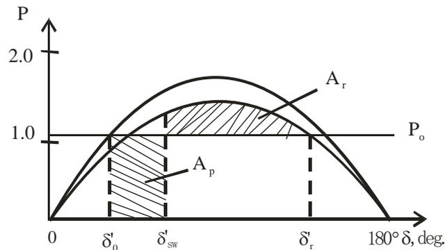
Figure 12.0 Generator swing curve
