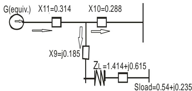
Figure 3.0 Simplified impedance diagram
