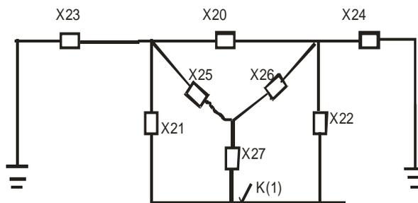
Figure 8.0 Conversion of Δ/Y impedance diagram
