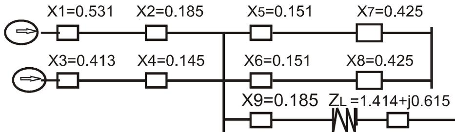
Figure 2.0 Impedance diagram of the transmission lines shown in figure 1
