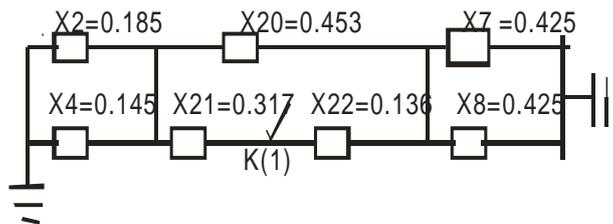
Figure 7.0 Zero sequence impedance diagram
