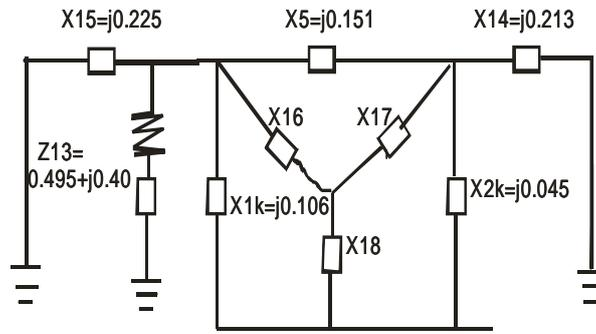
Figure 5.0 Δ/Y impedance conversion
