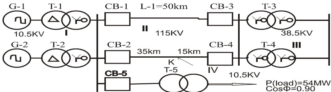
Figure 1.0 Circuit diagram of transmission lines
