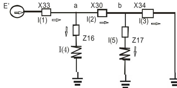
Figure 10.0 Equivalent generator circuit
