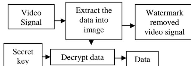
Fig:2 Block diagram of data retrieval process using watermarking
