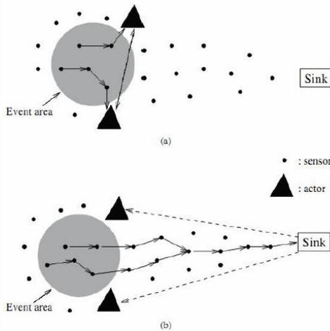
Fig. 1. (a) Automated and (b) semi-automated architecture of WSANs [3]
