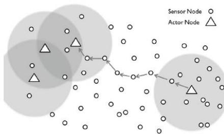
Fig.3 An isolated actor finding a path to other actors through sensor nodes
