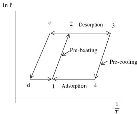
FIG.1 THE IDEAL ADSORPTION COOLING CYCLE
