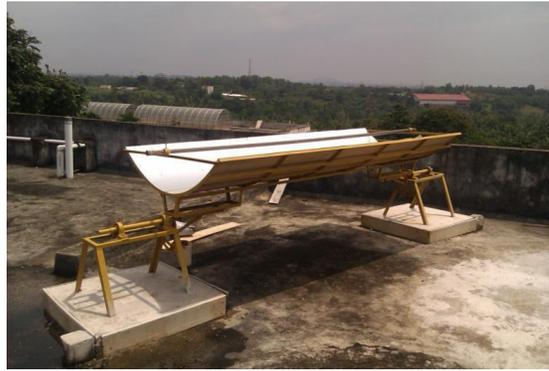
FIG. 2 PHOTOGRAPH OF THE PARABOLIC COLLECTOR
