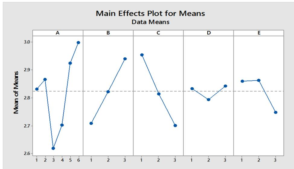
Figure. 2 Main Effect Plot for S/N ratio and MEAN for surface roughness
