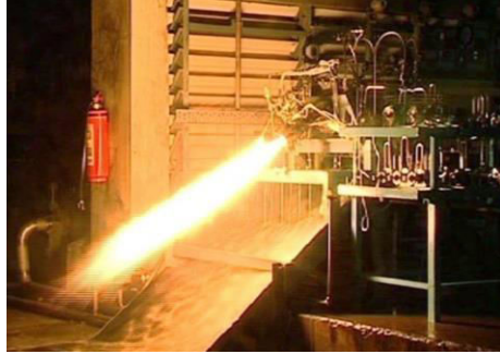
Fig 10 Single element Thrust chamber hot test
