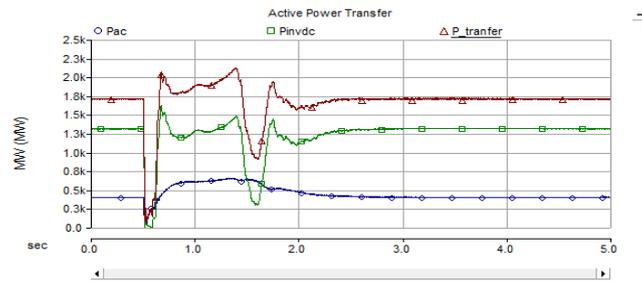
Fig. 11h. Ac (Pac), dc (Pinvdc) and total (P\_transfer) power transfer.
