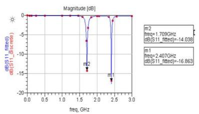
Fig.3.Return loss obtained at 1.7GHz and 2.4GHz
