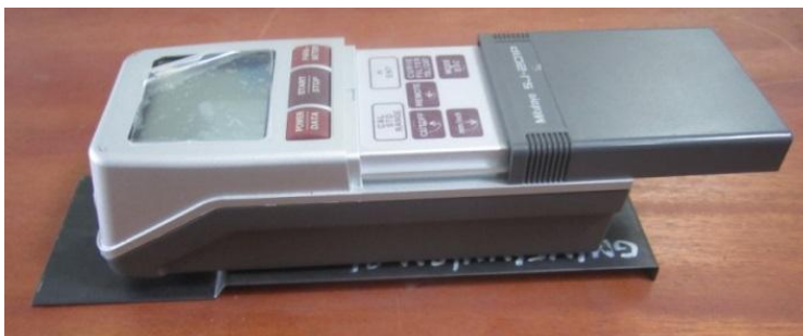
Figure 3: Talysurf (Surface roughness tester)
