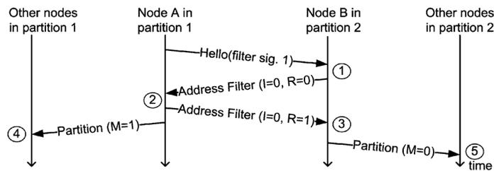
Fig. 6: FAP Scheme for Partition detection and merge
