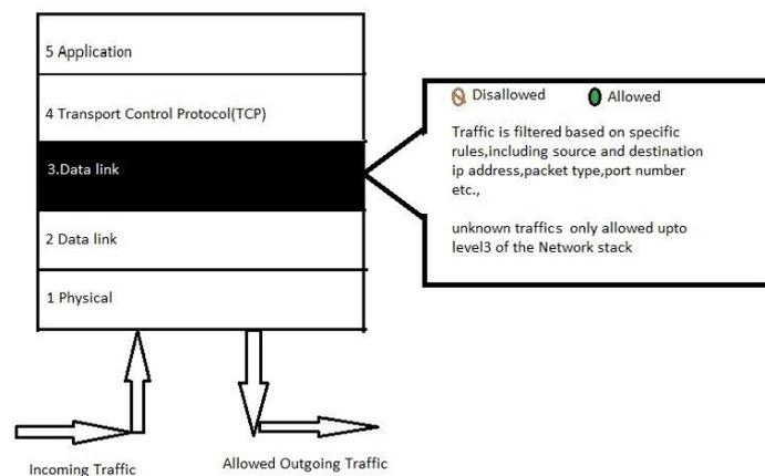
Fig. 1: Filtering of Traffic at different layers
