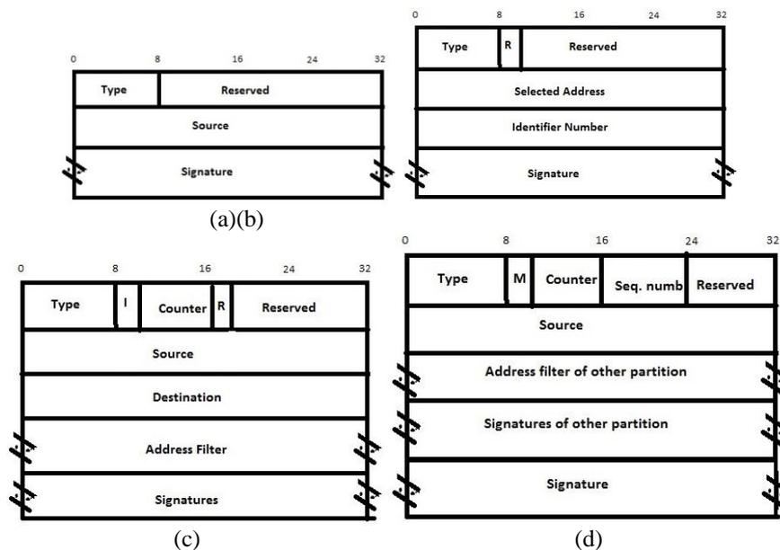
Fig 4: Messages for FAP for initialization, node joining, and partition merging (a) Hello (b) AREQ (c) AF (d) Partition
