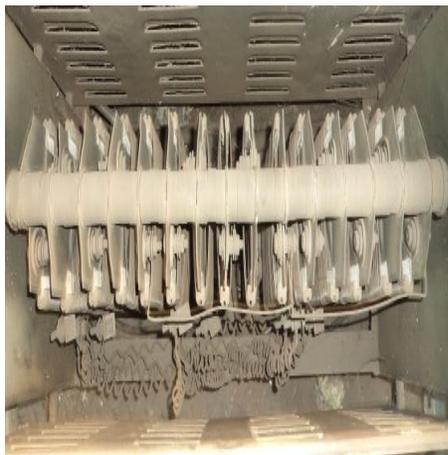
Fig.12-a Resistance connected to slip rings
