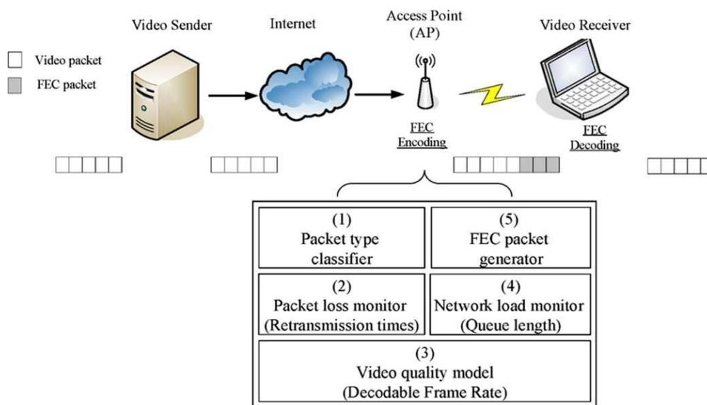
Fig. 4. Architecture of ERED-FEC controller.
