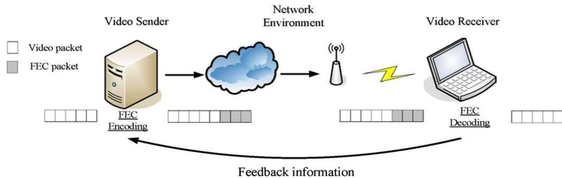
Fig. 2. Sender-based FEC scheme.
