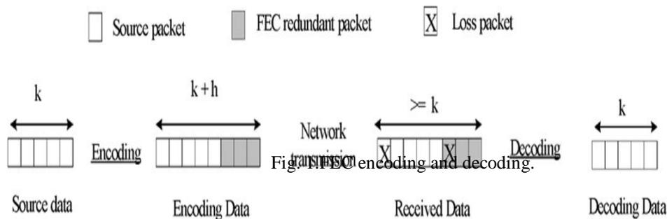
Fig. 1. FEC encoding and decoding.
