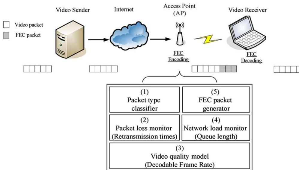
Fig. 4. Architecture of ERED-FEC controller.
