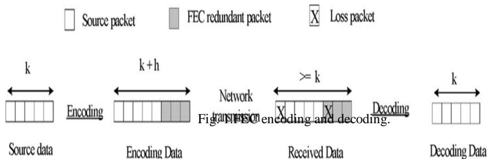
Fig. 1. FEC encoding and decoding.
