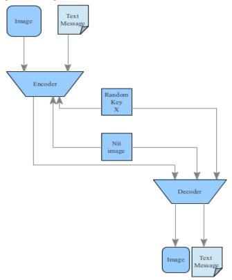
Fig. 3.2 Nit Process entire flow
