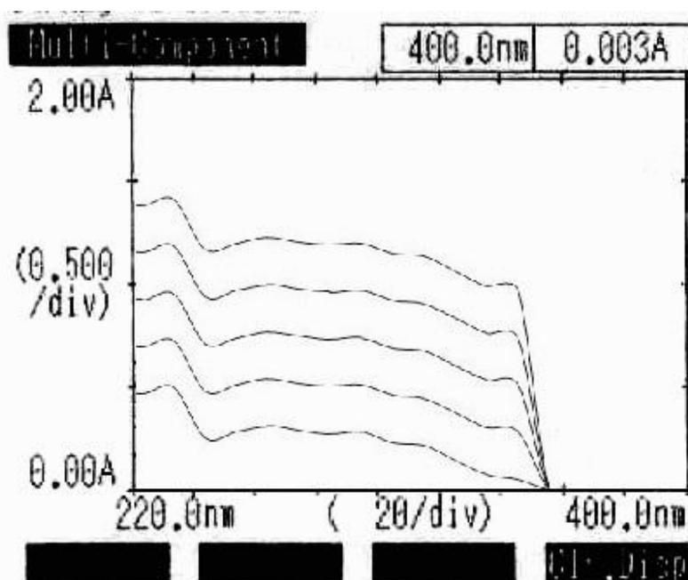
Figure 3: Overlain spectra of mixed standards of Telmisartan (TEL) and Hydrochlorothiazide (HCTZ).
