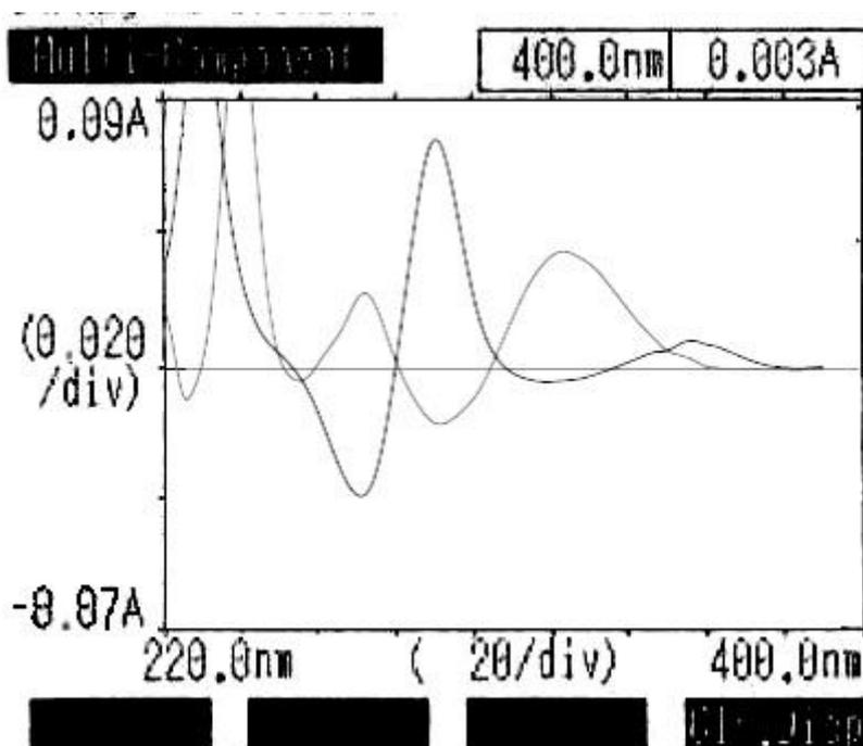
Figure 2: First Order Derivative spectra of Telmisartan (TEL) and Hydrochlorothiazide (HCTZ).
