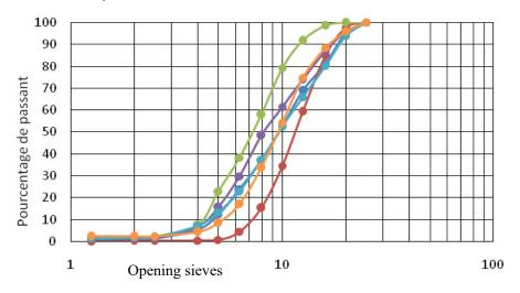
Figure 4. Particle size curves of lateritic nodules [11].
