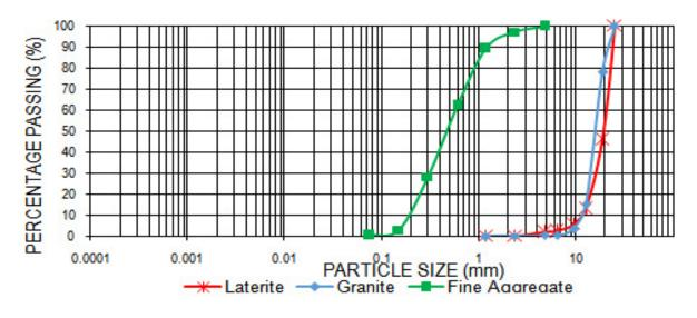
Figure 3. Particle size curves of lateritic nodules [6].
