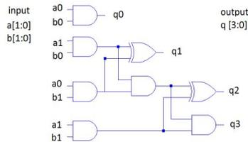
Figure 2: Hardware Realization of 2x2 block
