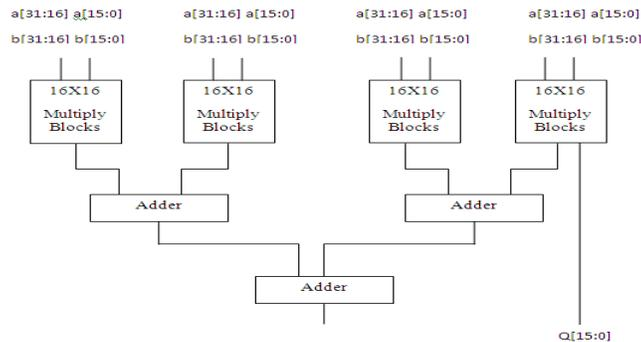
Figure 3: 32X32 Bits proposed Vedic Multiplier
