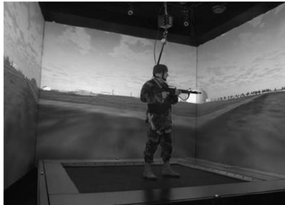
Figure 5. U.S. army research lab's omni-directional treadmill with CAVE.
