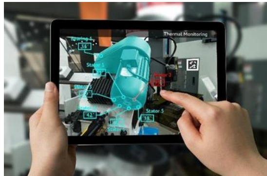
Figure 4. Thermal monitoring with augmented reality.
