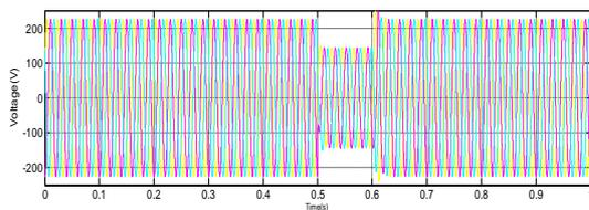
Fig. 3. Voltage Sag Waveform Without DVR
