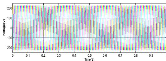
Fig. 4. Voltage Sag Waveform Compensated with DVR
