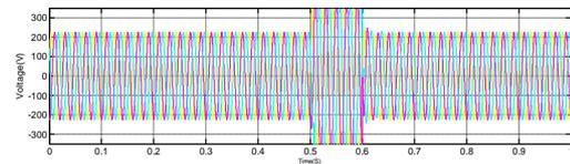
Fig. 5. Voltage Swell Waveform without DVR
