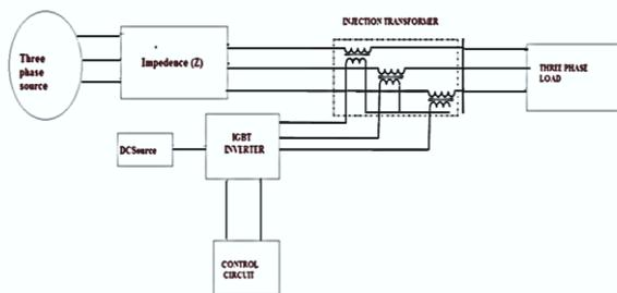
Fig.1. Three Phase Test System With DVR
