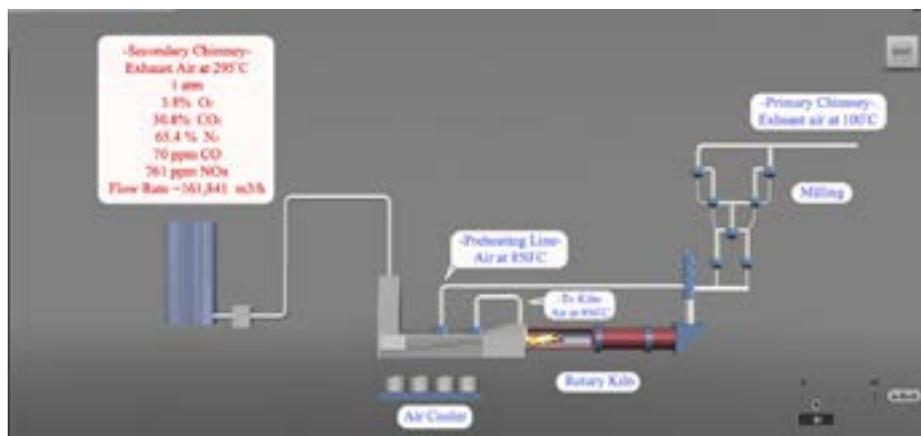
**Figure 2.** Factory layout with principal processes data.
