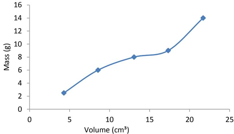
**Fig. 1 Density of Kankara clay using water displacement method**
