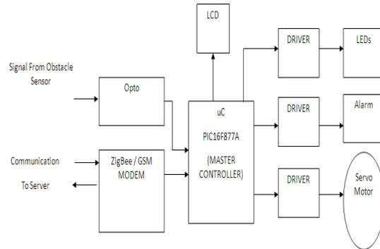
Fig 6.1 : Block Diagram of the Hardware to Control Unmanned Gate
