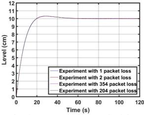
Fig. 6.System response with the MBC technique.
