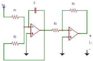
Fig. 2. Eletronic circuit that simulate a tank level system.
