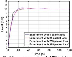
Fig. 5.System response without the MBC technique.
