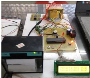
Fig : System of token generator using CC2500
