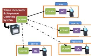
Figure2- Token Generator & Sequence Updating system
