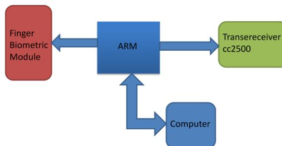
Figure shows the basic Block Diagram of the history tracker system which contains the finger biometric module attached with the ARM 7 Family Microcontroller (LPC2148). This is advanced controller nowadays.
