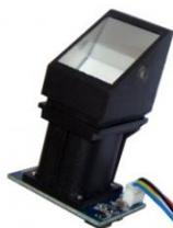
Figure 3. Finger Biometric Module
