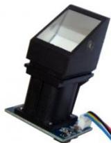
Figure 3. Finger Biometric Module
