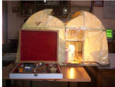
Figure 8: Laboratory model of polyhouse employed as a test bench
