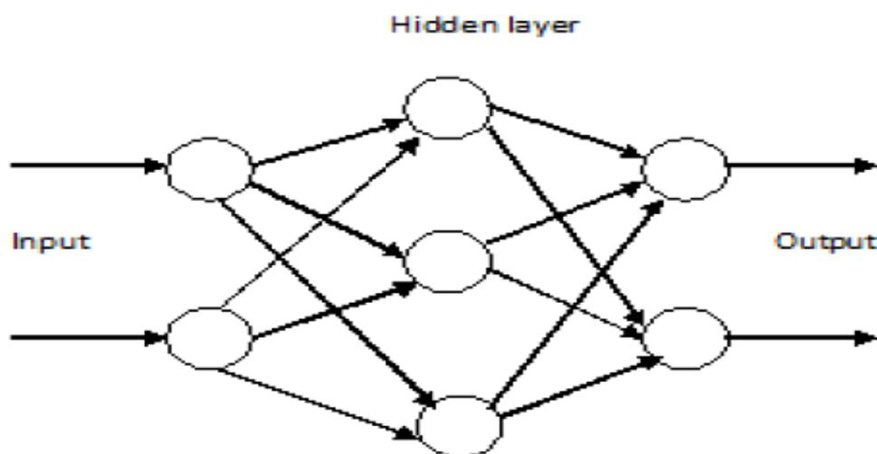
Fig.1. An example of a feed forward neural network
