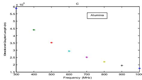
Fig. 4. Directional coupler length  $l$  versus frequency for alumina at -10(dB), coupling.
