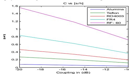
Fig. 2.  $s/h$  versus coupling level for alumina, Teflon, RO4003, FR4, and RF-60.
