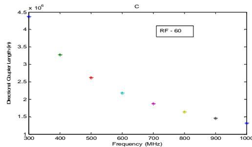
Fig. 8. Directional coupler length  $l$  versus frequency for RF-60 at -10(dB), coupling.
