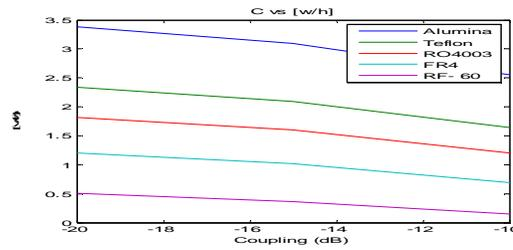
Fig. 3.  $w/h$  versus coupling level for alumina, Teflon, RO4003, FR4, and RF-60.
