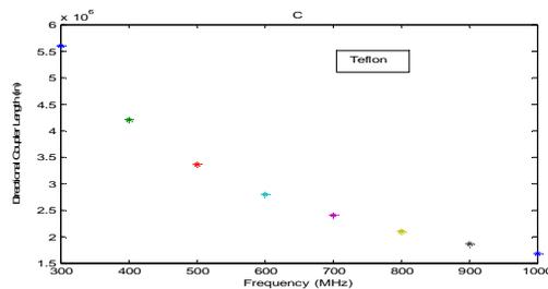
Fig. 5. Directional coupler length  $l$  versus frequency for Teflon at -10(dB), coupling.
