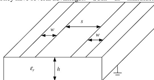
Fig 1. Two-line microstrip directional coupler
