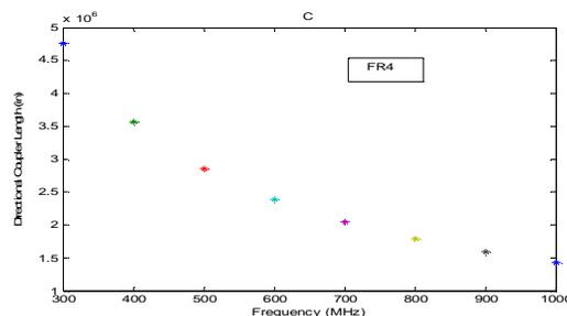
Fig. 7. Directional coupler length  $l$  versus frequency for FR4 at -10(dB), coupling.
