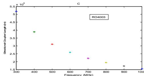
Fig. 6. Directional coupler length  $l$  versus frequency for RO4003 at -10(dB), coupling.
