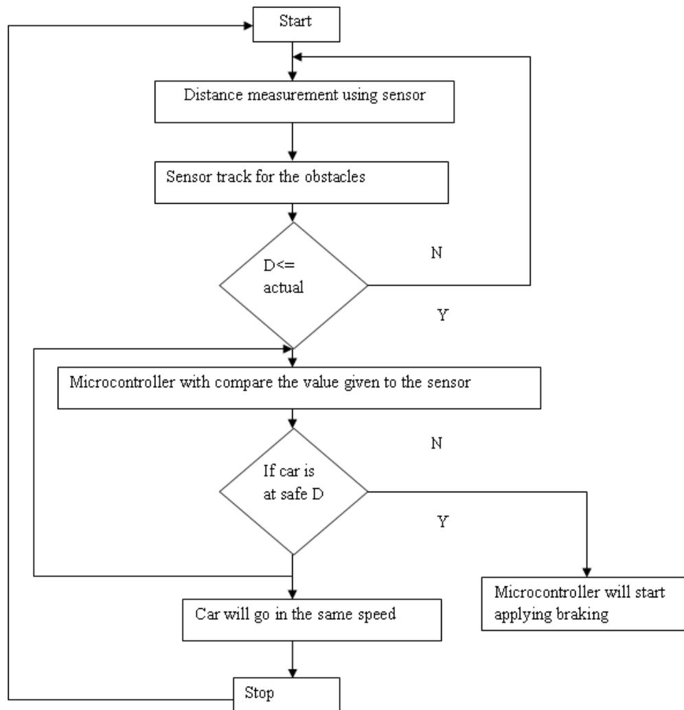
Fig. 5 Flow diagram of detecting obstacle
