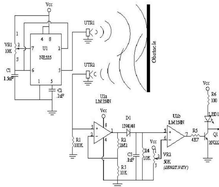
Fig. 4 Circuit diagram of ultrasonic sensor
