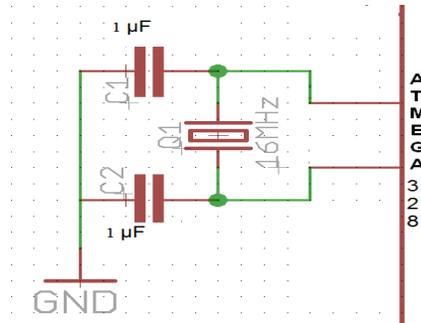
Fig. 3 Clock circuit
