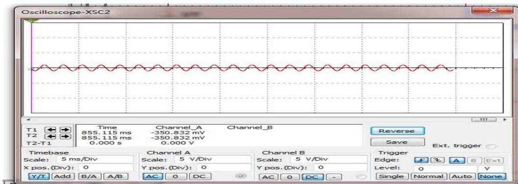
Fig 10: Input Waveform of AM Receiver Amplifier.
