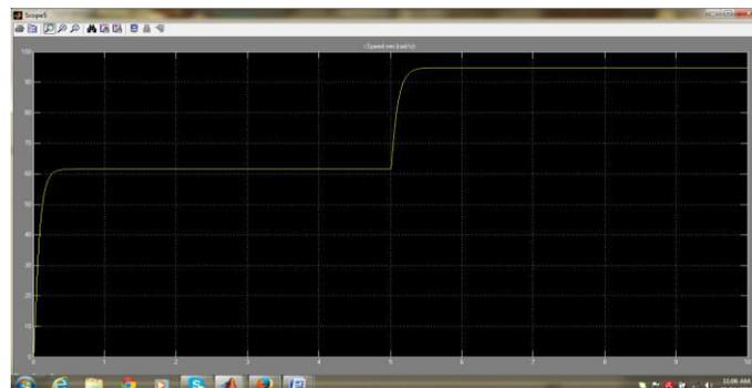
Fig. 3 Speed output of proposed Bi-Directional DC-DC converter with PI controller
