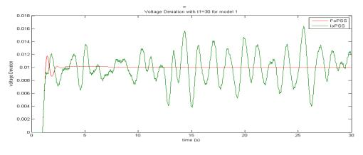
Fig 4Voltage deviation without an AVR when D = 2,  $\tau_1 = 30$ ,  $\tau_2 = 1$
