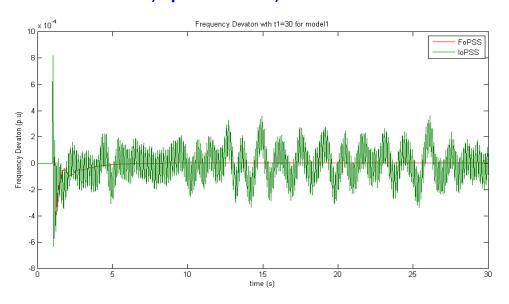
Fig 3 Frequency deviation without an AVR when D = 2,  $\tau_1 = 30$ ,  $\tau_2 = 1$
