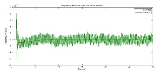
Fig 2 Frequency deviation due to 0.05 p.u. step change in both  $V_{ref}$  and  $T_m$  when D = 2,  $\tau_1 = 30$ ,  $\tau_2 = 1$
