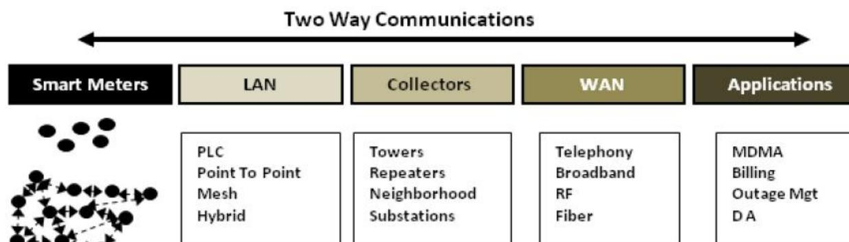
Fig. 3: Smart meter system Basic Architecture
