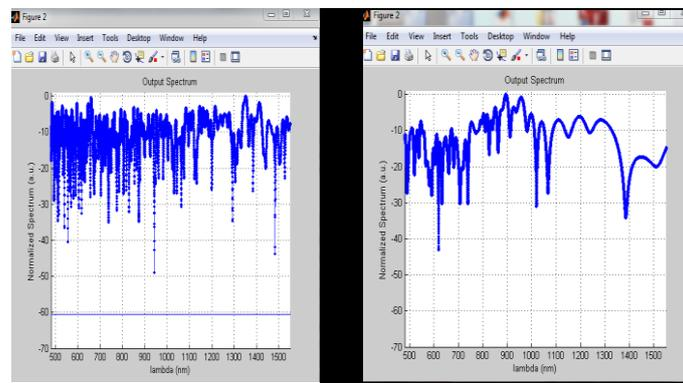
Fig1.15 SC pulse in PCF with  $\lambda=800$ ,  $l=0.0001\text{km}$  but value of peak power for left pulse is 10000W & for right pulse is 1000W.
