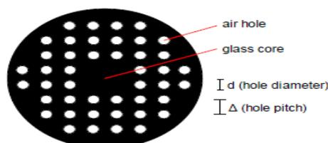
Figure 1.1: Cross-section of a common index-guiding photonic crystal fiber.
