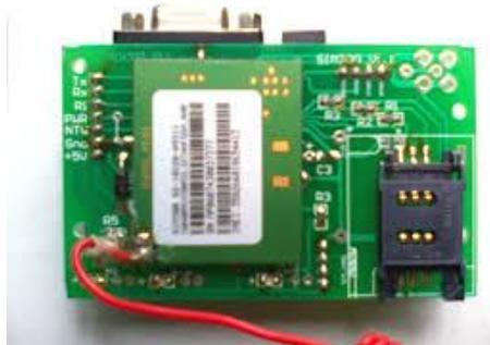
Fig. 5 Top view of GSM
