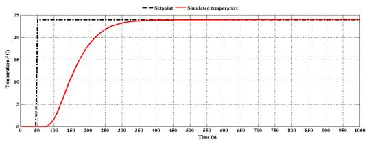
Fig. 7 Simulation of step response obtained by PI-intelligent in closed loop.
