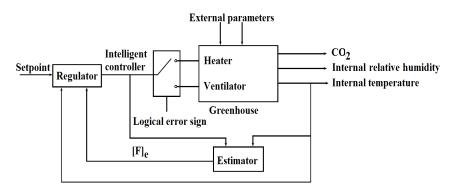
Fig. 8 Structure of the control system.
