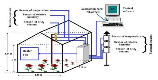
Fig. 1 Schematic view of the greenhouse system.
