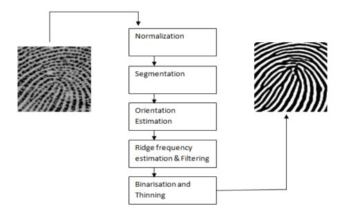
Fig 3.2 flow diagram of fingerprint enhancement
