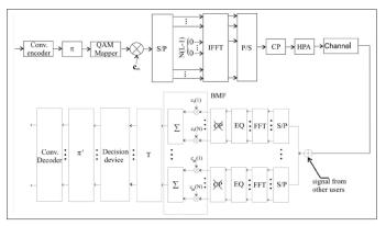
Fig 3.2 Block diagram Of MC-CDMA Communication System
