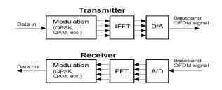
Fig 2.1 Block diagram of OFDMA Transmitter and Receiver
