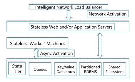
Fig. 15 Inbound Connectivity with Load Balancer
