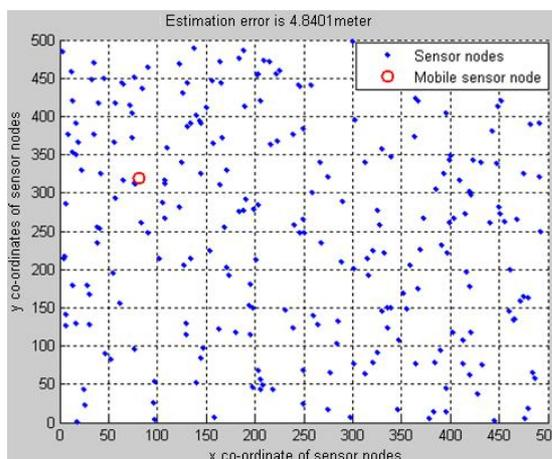
Fig. 2. Plot with 250 sensor nodes and its estimated error for unknown sensor nodes
