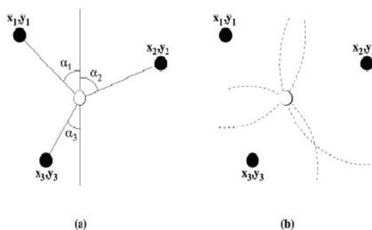
Fig1.a) Unknown location is found using three angle measurements (AoA) b) Unknown location found using the intersection of the radial measure from three known nodes(ToA)
