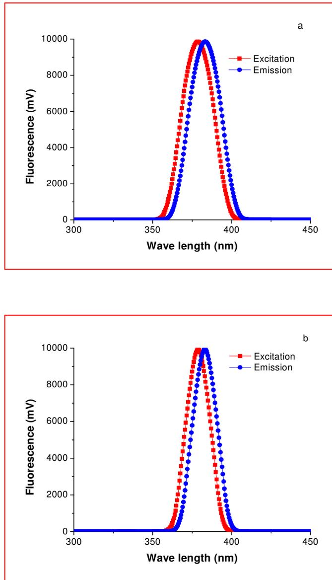
Fig .5. PL emission and excitation spectrum for a) TiO<sub>2</sub> and b) Hes-TiO<sub>2</sub>
