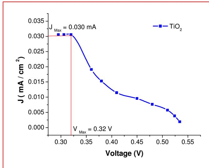
Fig .6. J-V Characteristic of TiO<sub>2</sub> nanoparticles
