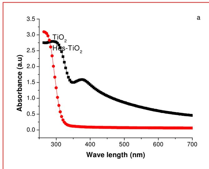
Fig .3. Absorption spectrum for TiO<sub>2</sub> and Hes-TiO<sub>2</sub>
