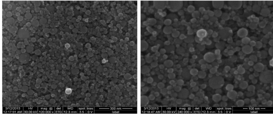
Fig .2. FESEM micrograph of the Hes-TiO<sub>2</sub>
