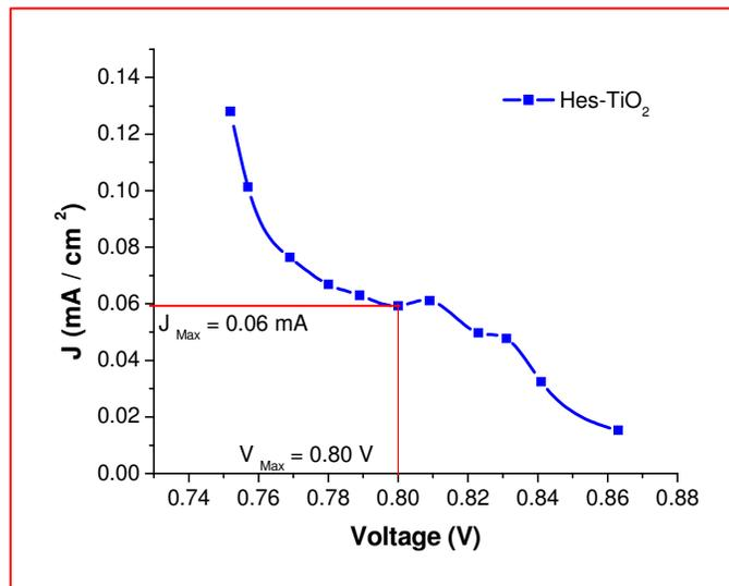
Fig .7. J-V Characteristic of Hes-TiO<sub>2</sub> nanoparticles
