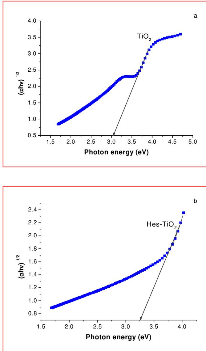
Fig .4. Direct and allowed band gap Extrapolation for a)  $\text{TiO}_2$  and b)  $\text{Hes-TiO}_2$
