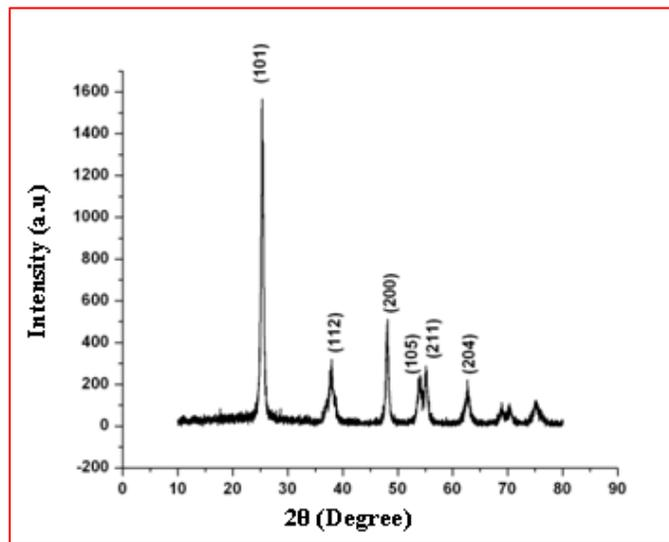
Fig.1 XRD spectrum for Hes-TiO<sub>2</sub>
