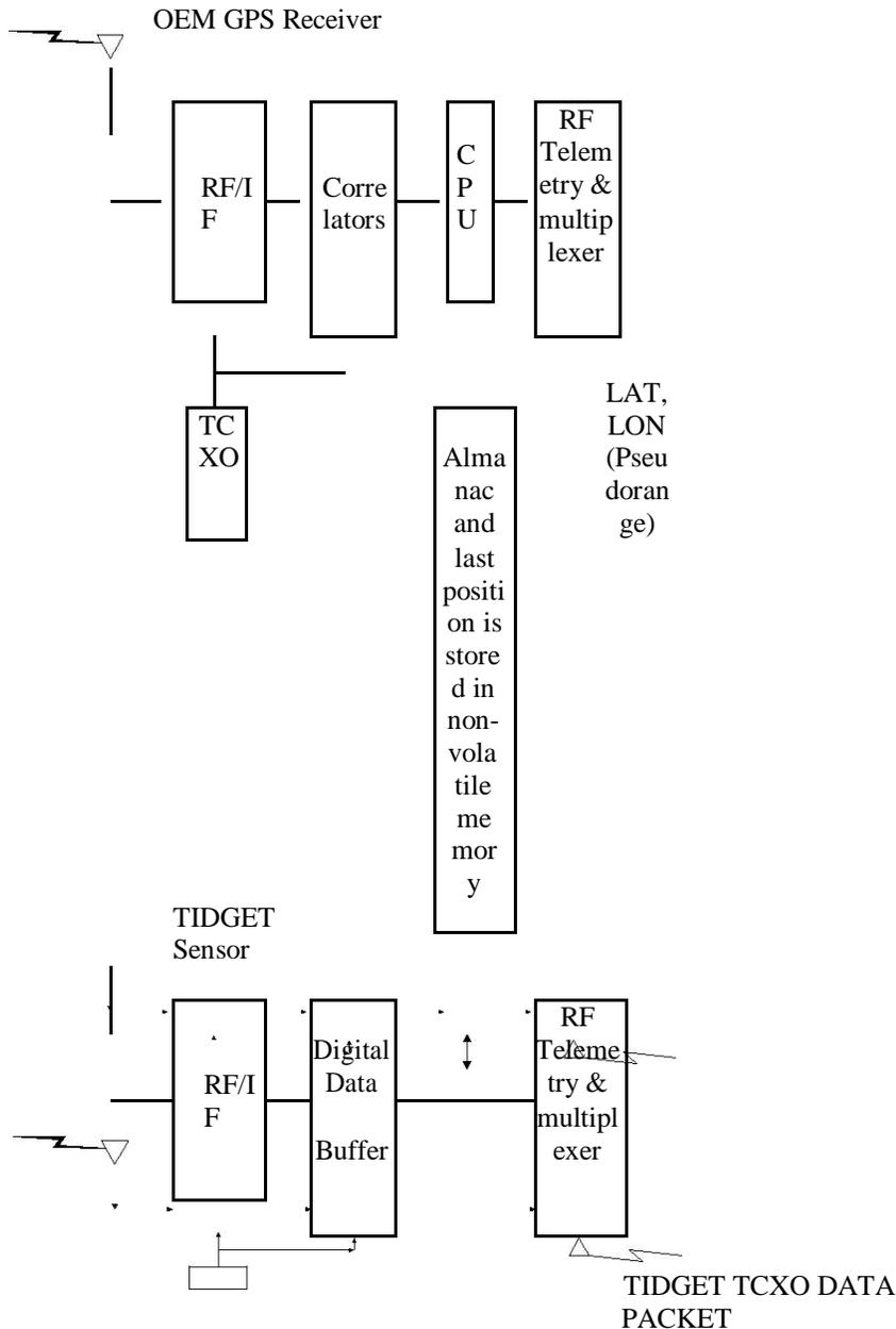
Figure 2 TIDGET Sensor
