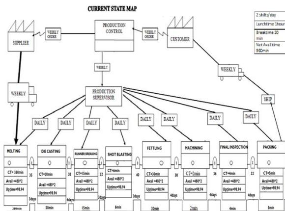
The daily demand for each parts & the cycle time and number of operators for every machine are noted. Then the productions of each machine are calculated. These are tabulated in fig.3
