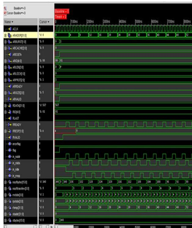
Figure 4: Increment Address for Read Operation
