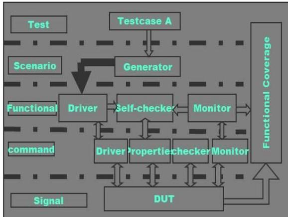
Figure 2: layered based verification environment.
