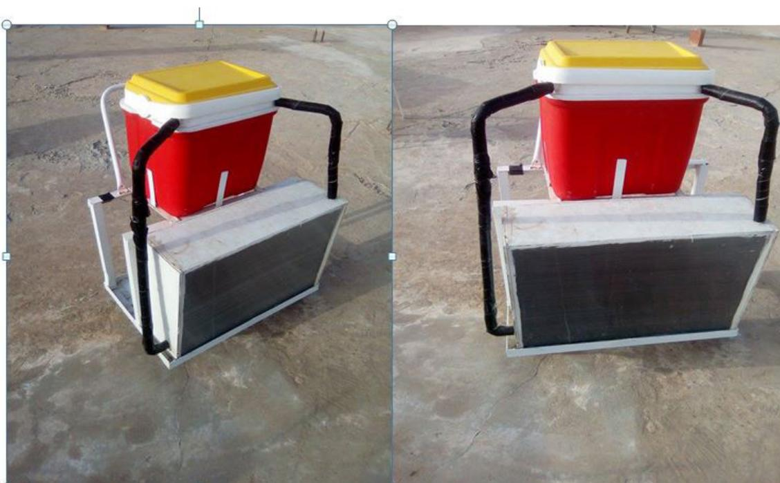
Figure 4. Wall solar water heater to thermosiphon "ThWSWH" according to two different view.
