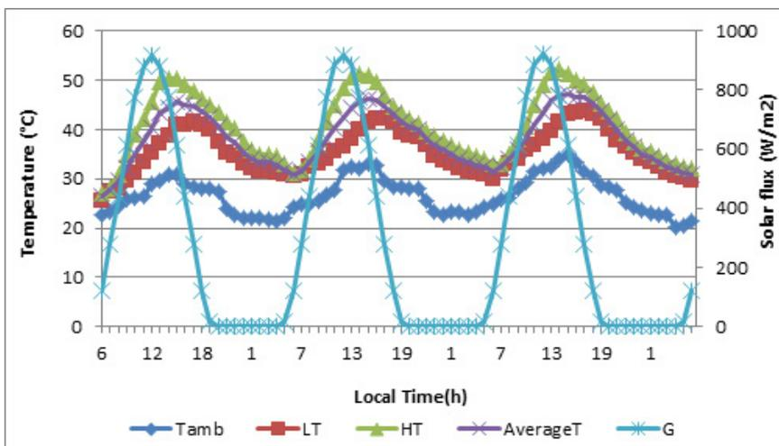
**Figure 7.** Variation of the incident solar flux, the ambient temperature, the temperature high, low temperature and the average temperature of the water in the storage tank in the ThWSWH according to the local time during three successive days (9-10-11/07/2017).
