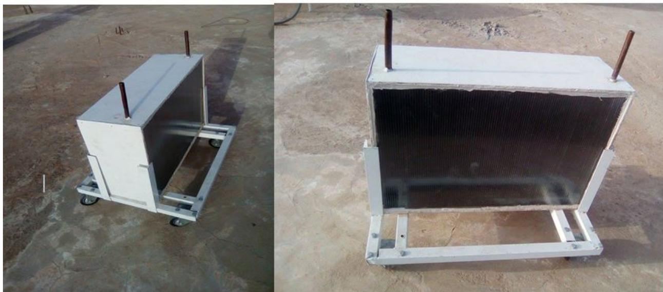
**Figure 1.** Wall solar water heating to integrated storage according to two different views (IWSWH).
