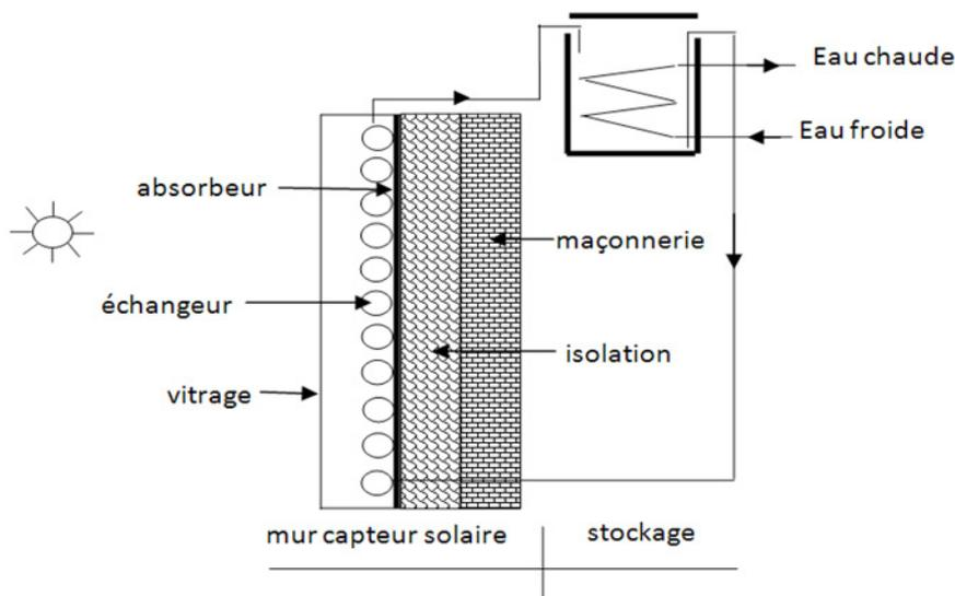
Figure 3. Block diagram of a wall solar water heater to thermosiphon.
