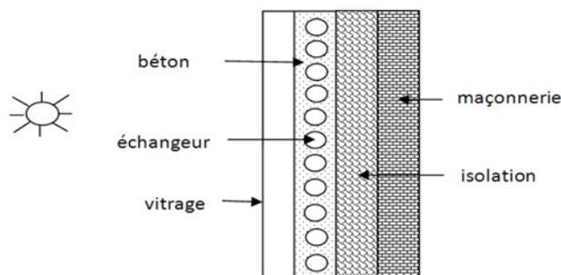
**Figure 2.** Block diagram of the wall solar water heater to integrated storage built in.
