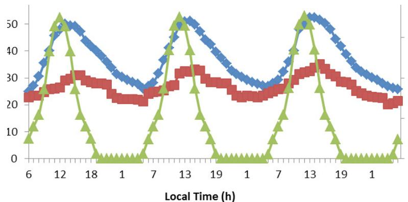
**Figure 5.** Variation of the incident solar flux, the ambient temperature and the temperature at the outlet of the water of the IWSWH according to the local time during three successive days (9-10-11/07/2017).
