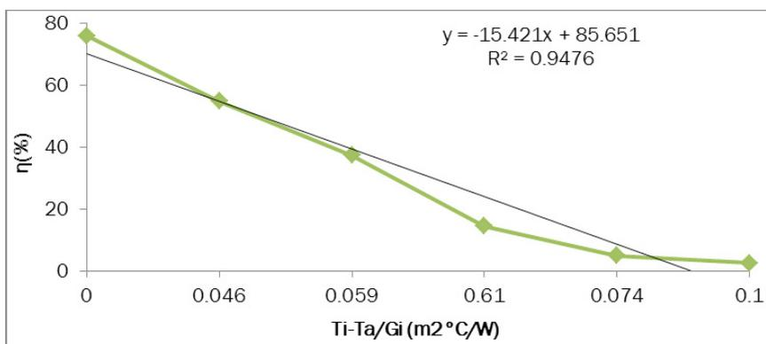
**Figure 6.** The effectiveness of the IWSWH according to standardized gain during the day of the test (9/07/2017).
