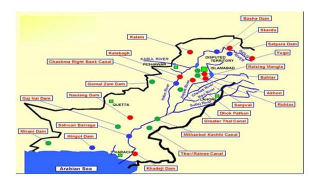
Economic utilization for the hydropower potential in Pakistan is relatively 20,000 MW. Many hydropower plants have been developed at various areas of Pakistan in 1998 of about 4,825 MW, at Warsak 2,40 MW, at Tarbela 3,478 MW, at Mangla 1000 MW as well as small hydropower plant on Canals with capacity 107 MW (Figure 5). Figure 5. Hydroelectric power generation system.
