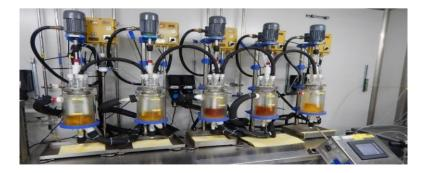
Agitation reactors are based on the principle of continuous stirred tank reactors. It features a reaction block which is mounted on the agitator <sup>[15]</sup>. The agitation reactor utilizes freely moving agitator within the reactor block. The
