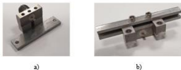
Figure 5. Custom made SMA connectors for a) microstrip and b) for CPW application.
