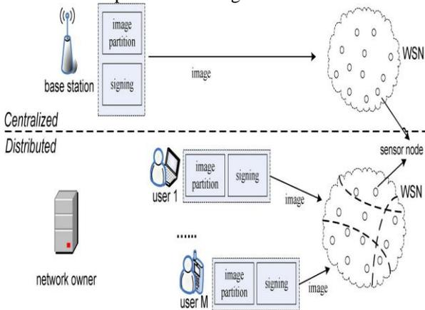
Fig. 1. system overview of centralized and distributed reprogramming approaches
