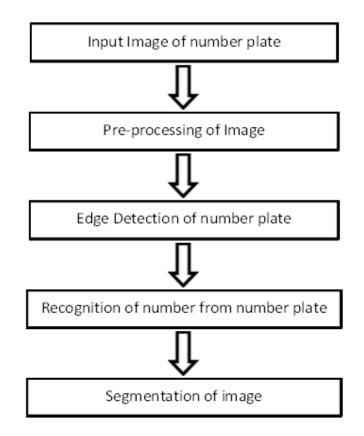
Figure:1 A Automated Number Plate Recognition (ANPR).
